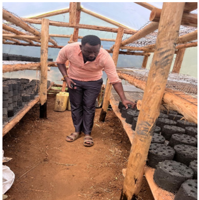
Figure 9: One of the solar housings for briquette drying in Kikuube district under the clean energy hub.
